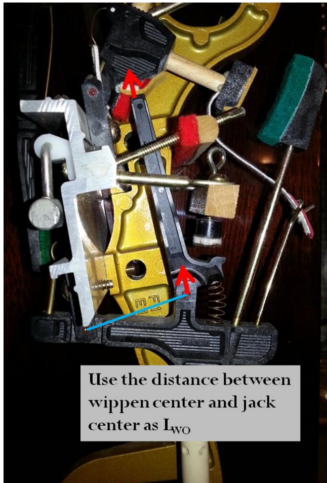
Photo 5: Determining output length of the wippen.
