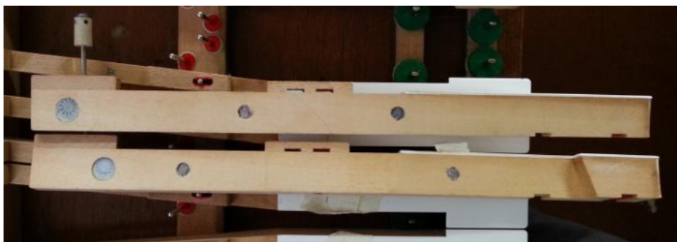
(Fig 6) Added key leads to both side of key stick at same distance from balance hole
