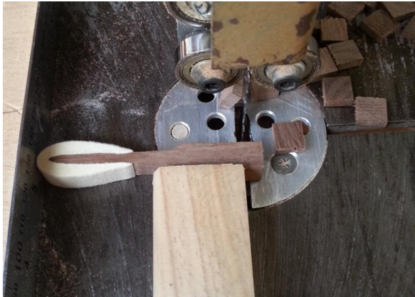
(Fig 9) Cutting hammer tail on a band saw. With new hammers shorten the tail before gluing.
