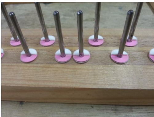
(Fig 14) Cut punching cloth which is glued to thin paper washer (pink in the photo)
