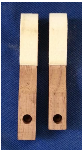
(Fig 10) Shortened hammer tail (Left: original, Right: shortened.)
