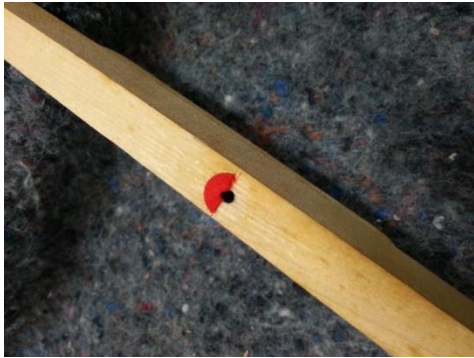
(Fig 13) Cut punching cloth glued to the key
