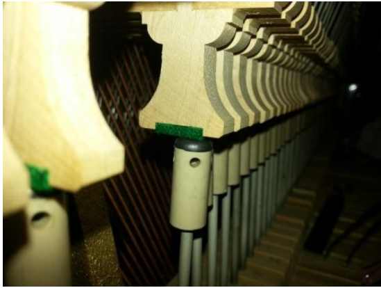
(Fig 12) Pilot is set forward by 3mm from the centre of the heel cloth,
